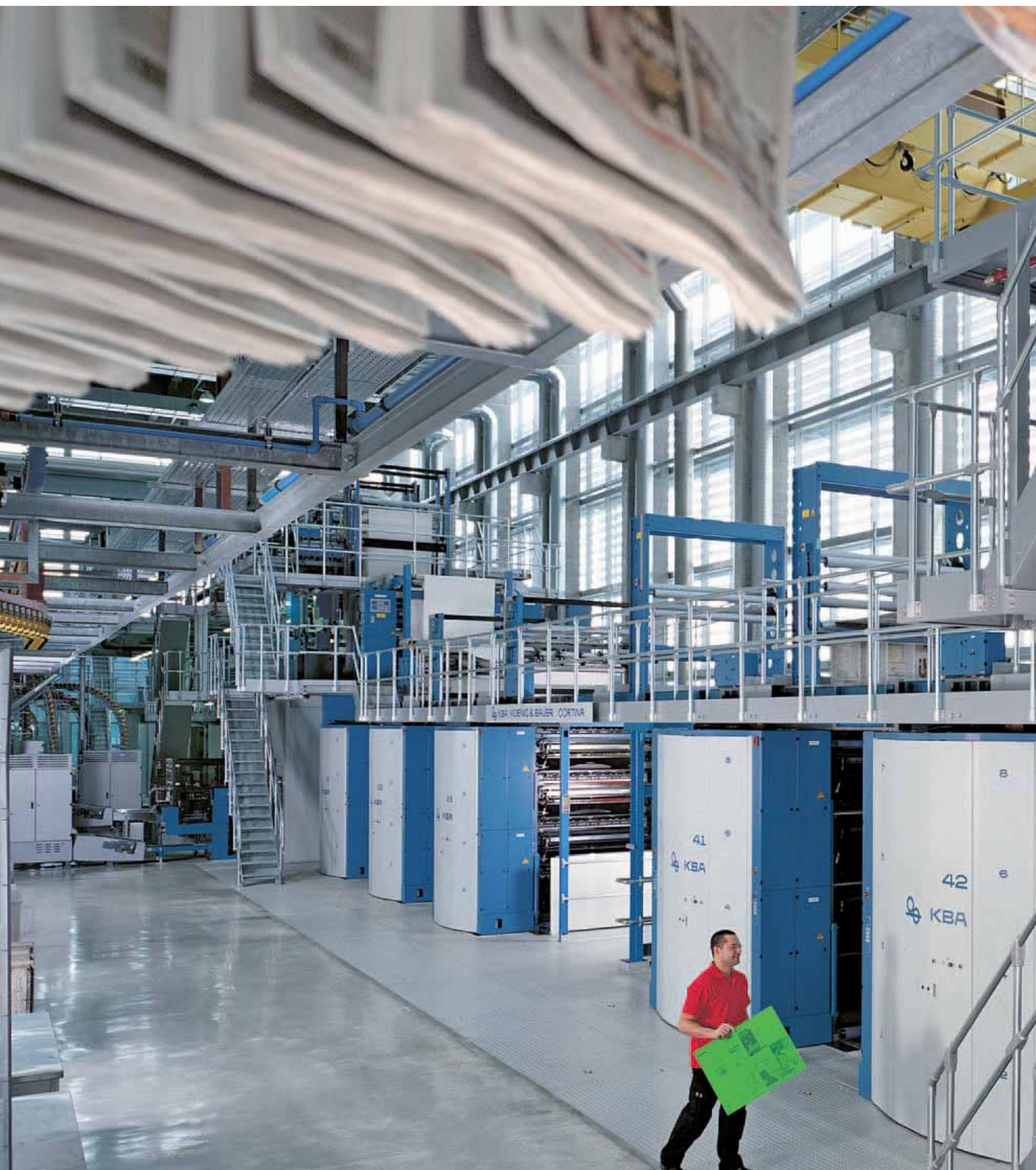
Multi-unit Cortina press line for the environmentally friendly production of newspapers and semi-commercials at de Persgroep's Eco Printing Center in Lokeren, Belgium
