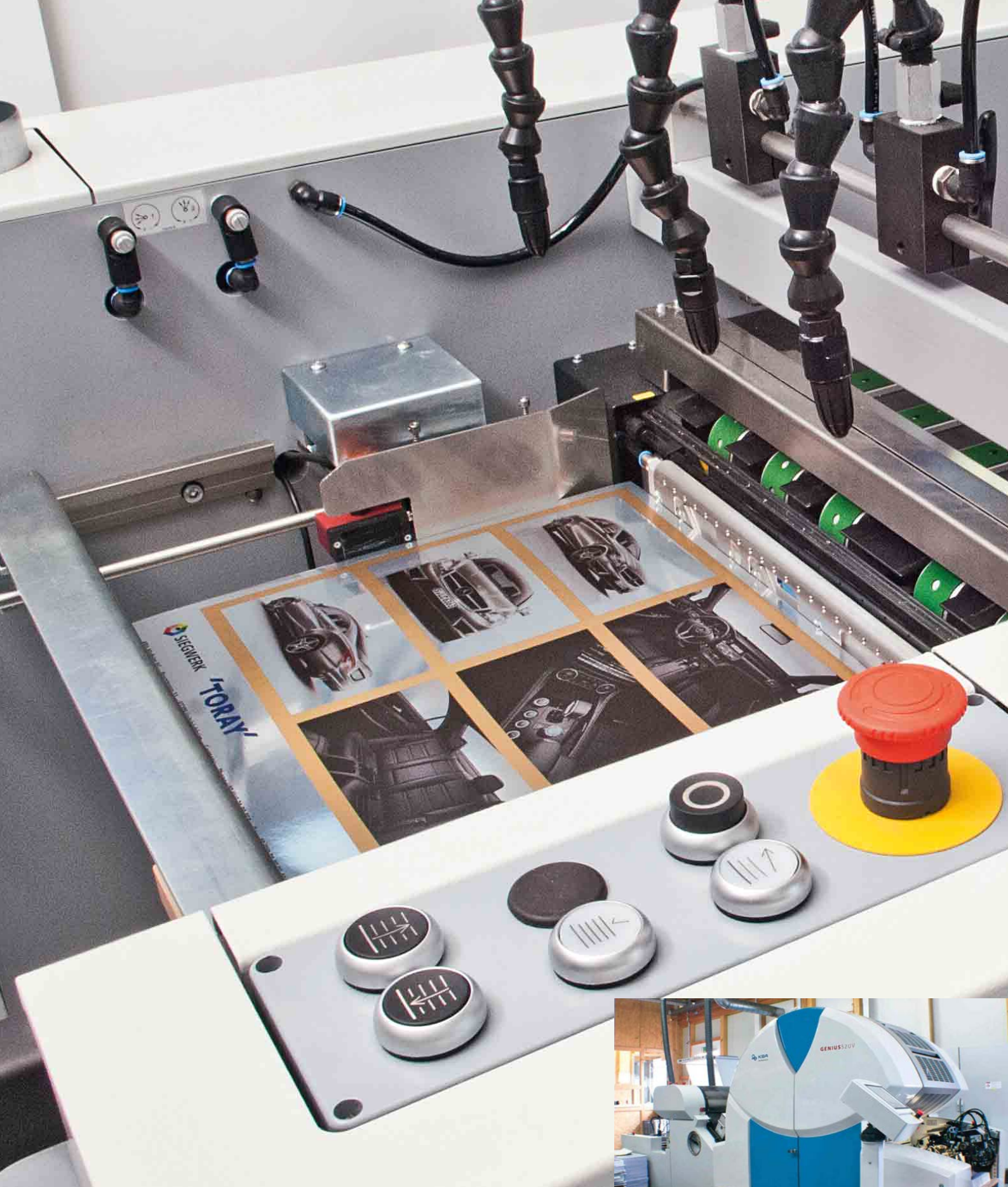
The small-format waterless Genius 52UV offset press from KBA-MePrint prints smart cards, foils, stickers and many other advertising products on comparatively expensive substrates. This press services a premium quality niche market
