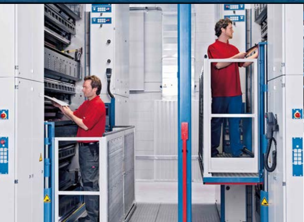
Newspaper printing means time pressure: the highly automated compact Cortina and Commander CT web presses (photo) ensure rapid edition changes. New plates can be inserted into the automatic plate changers while the press is still running
