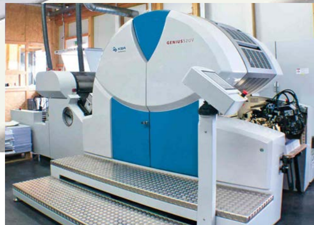
The small-format waterless Genius 52UV offset press from KBA-MePrint prints smart cards, foils, stickers and many other advertising products on comparatively expensive substrates. This press services a premium quality niche market
