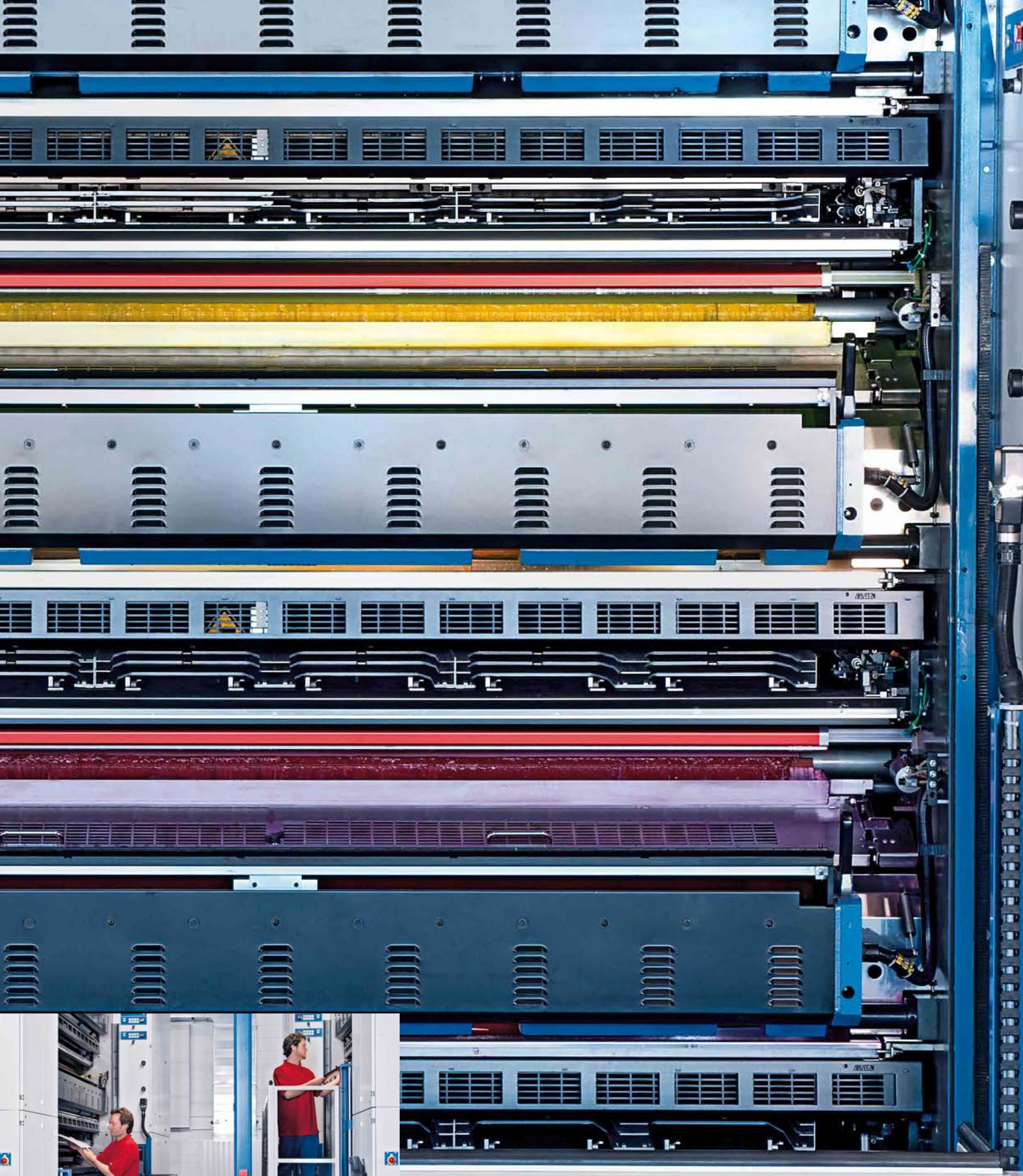
Newspaper printing means time pressure: the highly automated compact Cortina and Commander CT web presses (photo) ensure rapid edition changes. New plates can be inserted into the automatic plate changers while the press is still running
