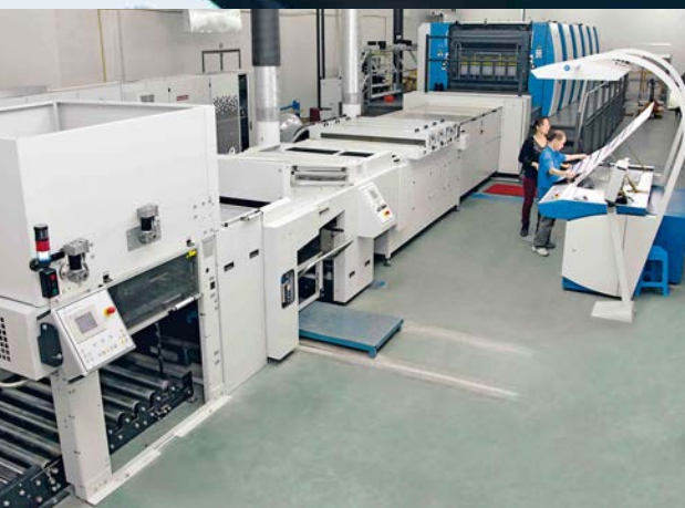
KBA-MetalPrint in Stuttgart has a strong footing globally in the metal-decorating market with the production of entire printing, coating and drying lines. The photo left shows one of several MetalStar presses in action at our user China Food Packaging
