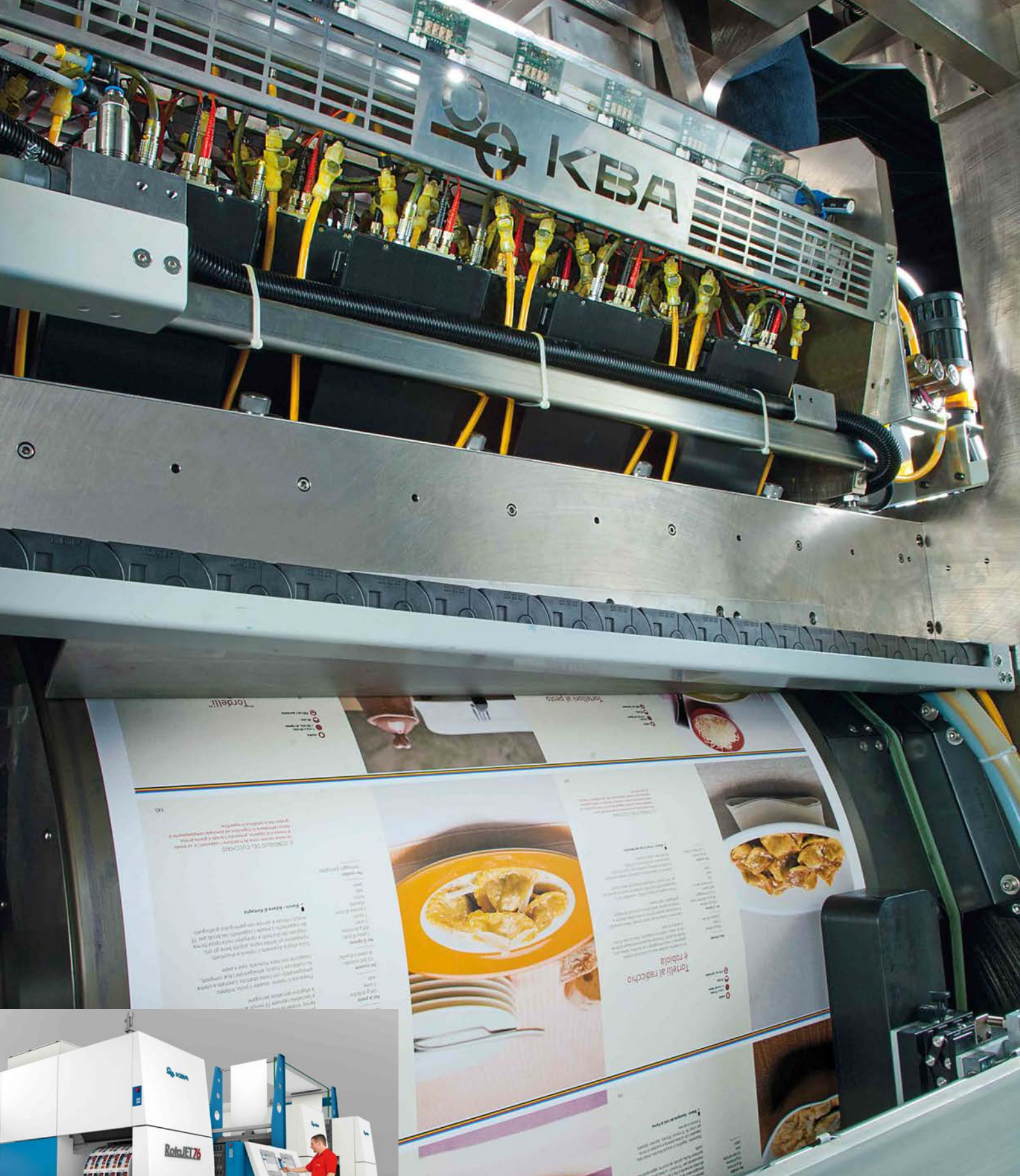
The new KBA RotaJET 76 digital printing press, developed and produced at our main plant in Würzburg, addresses the growing market for short-run colour and personalised print products. Initially our focus is on the book, direct mail, advertising, newspaper and magazine sectors
