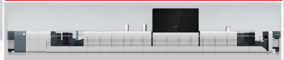
Perfector presses with printing units and coaters before and after the perfecting unit add finishes that boost the attractiveness of folding cartons at the point of sale.
